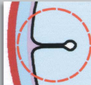
Channels are formed at the blind end of the infolded cuff-wall. Pharyngeal secretions don't enter the trachea at the area of contact between cuff- and tracheal-wall. Leakage takes primarily place by formation of tunnels inside the cuff-wall.
